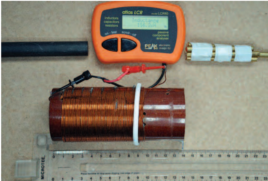
PHOTO 1: The experimental setup to measure the effects of a shorted turn, brass slug and ferrite rod on the inductance of a coil.
